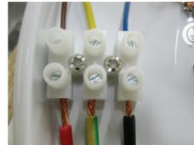
No insulating plate under the terminal block. Wire insulation stripped back too far.
