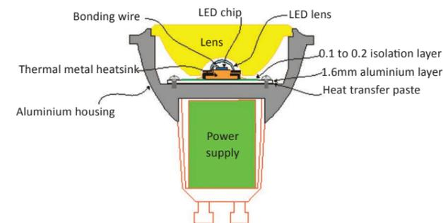
The basic requirement is that no single failure can result in dangerous voltage becoming exposed so that it might cause an electric shock and that this is achieved without relying on an earthed metal casing. This is usually achieved at least in part by having two layers of insulating material surrounding live parts or by using reinforced insulation such as insulating sleeves, grommets and bushings.
