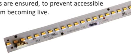
Because of the construction of LEDs, the LED chip emits directional light in a fairly narrow beam, whereas light from most traditional sources is omni-directional (emitting light in all directions in space) and most luminaires are designed for these light sources.
