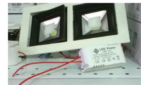
The non-compliant LED luminaire's driver (above) is marked with the double insulated marking, but the supply leads only have basic insulation and are not marked.
