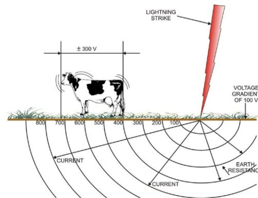
A surge is when the voltage or current increases suddenly to a value exceeding the rated value by a few percent (typically 10 to 20%) and falls back to normal in a few milliseconds (typically 20 to 30 ms). This is also referred to as a 'transient' and can be caused by switching power ON to un-energised transmission lines, during short circuits and arcing faults to earth. In the case shown, the voltage gradient between the front and back legs of the cow is high enough to electrocute the animal.
