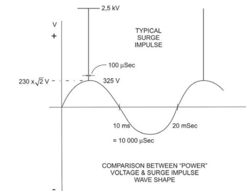
A typical voltage surge or spike has a peak of 2.5 kV with a 1.2 micro-second (1.2/1 000 000 of a second) rise time and a fall to 50 % of the peak value in 50 microseconds.
