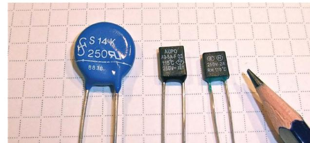
**The thermal disconnecter is a crucial component in the surge protection circuit as it prevents a fire developing within the MOV assembly after it has absorbed repetitive surges over its lifetime.**
