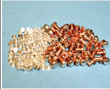
Where current is being connected and disconnected, it is essential that small silver or silver inlayed copper contact tips are part of the contact construction.
